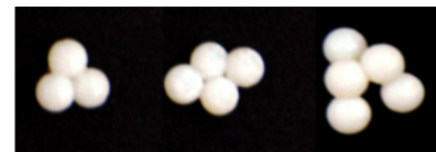
Fig. 2. ‘Granular Molecules’, each 3d-printed as one piece from hard plastic. Each sphere is ~3mm in diameter.
