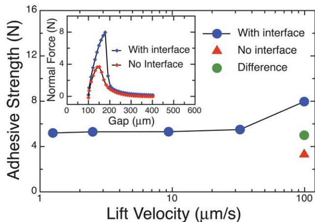
**Fig. 6** Lift speed dependence of the adhesive strength for a 40% CIP suspension in water at 100  $\mu\text{m}$  initial gap, 200 mT applied field, and 7.5 mm initial radius. Inset: normal force vs. gap for 100  $\mu\text{m s}^{-1}$  with and without the liquid–air interface.
