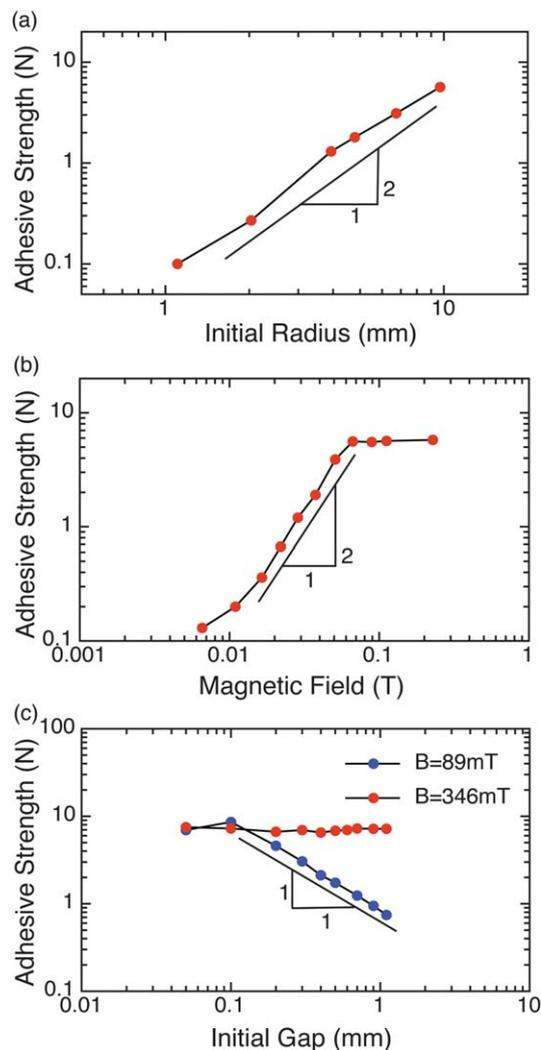
**Fig. 7** Scaling of the maximum adhesive force for a 40% CIP suspension in water. (a) Radius scaling (100  $\mu\text{m}$  initial gap, 1.25  $\mu\text{m s}^{-1}$  lift speed and 228 mT field). (b) Magnetic field scaling (100  $\mu\text{m}$  initial gap, 1.25  $\mu\text{m s}^{-1}$  lift speed and 7.5 mm initial radius). (c) Gap scaling for small and large applied field (100  $\mu\text{m}$  initial gap and 7.5 mm initial radius).
