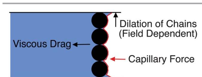
**Fig. 8** Sketch of a simple physical picture used to explain MR adhesion. Chains tend to dilate in the direction of the applied field and push against the upper and lower confining surfaces, resulting in a frictional anchoring force. To drag the chains inward as the top plate is lifted and the liquid recedes, either the capillary forces or a viscous drag have to overcome this anchoring force.
