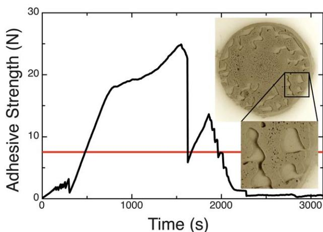
**Fig. 9** Adhesive force measured during drying without applied field for a sample initially consisting of 40% CIP in water (100  $\mu\text{m}$  fixed gap and 10 mm initial radius). The red line indicates the value of the adhesive strength given by  $2\gamma\pi R^2/a$ . Inset: image of the sample after drying (with zoomed-in detail).
