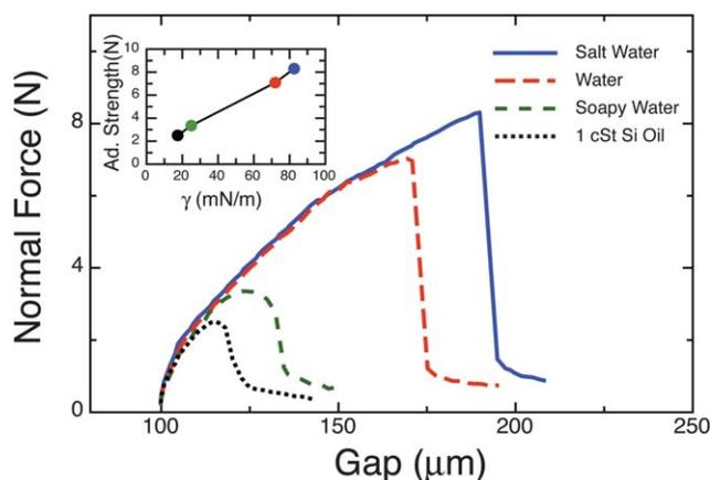
**Fig. 5** Effect of surface tension on the adhesive strength for a 40% CIP suspension in water at 200 mT applied field,  $1.25$   $\mu\text{m s}^{-1}$  lifting speed, and  $7.5$  mm initial radius. The measured values of the surface tension were:  $17.4$   $\text{mN m}^{-1}$  (1 cSt Si oil),  $72$   $\text{mN m}^{-1}$  (water),  $25$   $\text{mN m}^{-1}$  (soapy water),  $82.5$   $\text{mN m}^{-1}$  (salt water). Inset: dependence of adhesive strength on surface tension.
