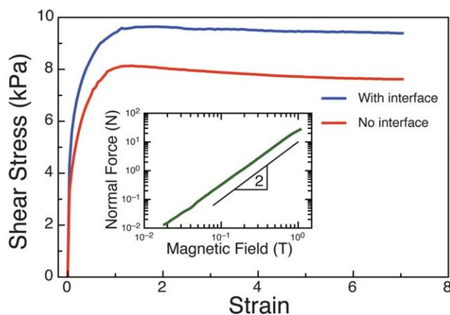
**Fig. 3** Stress vs. strain from shear measurements on a 40% CIP suspension in water at 200 mT applied field with and without the liquid-air interface. Inset: normal force *vs.* magnetic field at zero shear strain, with the liquid-air interface removed by flooding.
