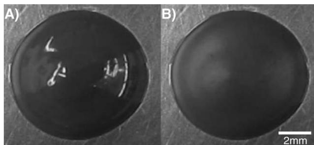
**Fig. 4** Top view of a drop of 40% CIP suspension in water. (A) No field applied. (B) Same drop with magnetic field applied from below.
