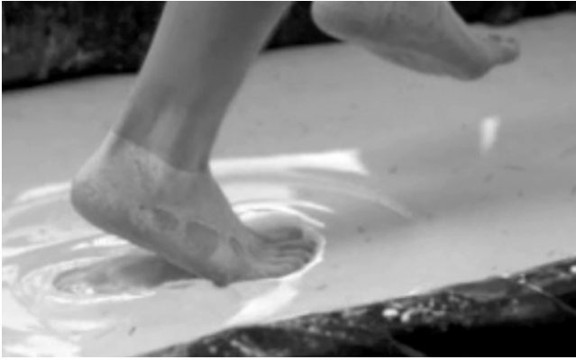
Figure 1. Snapshot of a person running on top of a pool filled with a dense suspension of cornstarch and water. The fluid can temporarily hold up the person's weight like a solid, sustaining stresses orders of magnitude beyond the capabilities of the suspending Newtonian liquid (here water). The suspension behaves liquid-like before and after impact, for example gravity waves are seen to propagate along the surface, and without running, the person would sink into the suspension as in a normal liquid.
