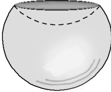
Figure 5. A ring ridge forms when a part of a spherical shell snaps through.
