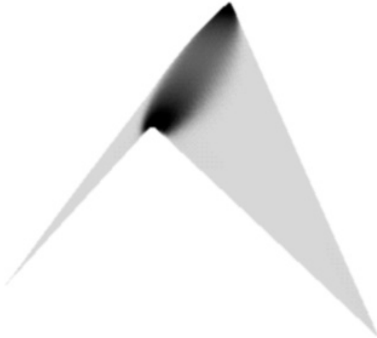
Figure 12. A kite shape made from a flat, rhombus-shaped surface by exerting normal forces on the perimeter sites. The forces constrain the perimeter to follow a rectilinear frame with dihedral angle \alpha equal to that of the tetrahedron, namely \cos^{-1}(1/3) . Ridge length is X = 100a and thickness is h = a/13.7 .
