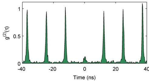
FIG. 4. (Color online)  $g^{(2)}(\tau)$  measurement under pulsed excitation taken at the frequency of one of the polariton peaks. The peak at  $\tau=0$  has an integrated area of  $21\% \pm 2\%$  the average area of the peaks at other times, demonstrating strong antibunching.
