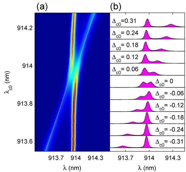
FIG. 3. (Color online) (a) Measured density plot of the spectra as the cavity mode is tuned into and out of resonance with the quantum dot exciton.  $\lambda_{c0}$  is the uncoupled mode wavelength. The dashed lines are the calculated peak positions which agree well with the measured positions. (b) Individual spectra at different values of  $\Delta_{c0}$ , the uncoupled cavity mode detuning from resonance in nm.
