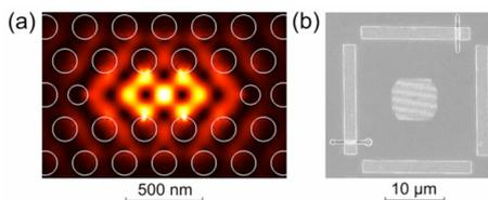
FIG. 2. (Color online) (a) Simulated electric field intensity in the modified  $L3$ -type cavity. The color scale goes from black (zero) to white (maximum intensity). (b) SEM image of a photonic crystal positioned near the center of a set of four gold markers. The lines on the upper and left markers are due to the detection procedure of the electron beam writer.
