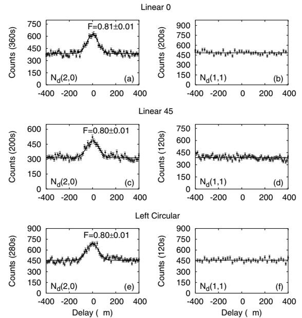
FIG. 2. Experimental data demonstrating cloning on a beam splitter.  $N_d(2, 0)$  increases as the photon wave packets overlap, while  $N_d(1, 1)$  remains the same. The data on the left are fitted to a Gaussian and the fidelity, displayed in each plot, is deduced from the fit as described in the text.
