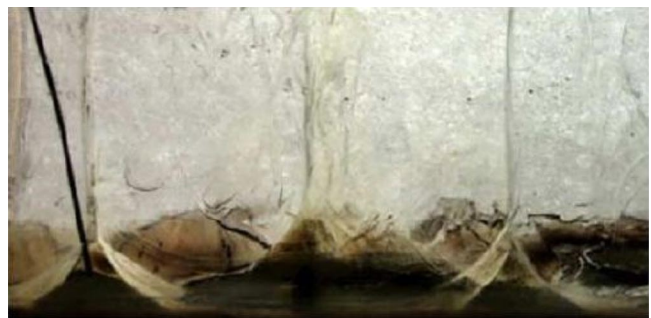
FIG. 1 (color online). Axisymmetric tendrils entrained by a warmer, upwards flow in a 2-layer thermal convection experiment with miscible oils. Convection is driven by heating the bottom of the tank and cooling the top. The lower fluid is less viscous than the upper, and the spacing between tendrils is O(10\text{ cm}) . The dark vertical line on the left is a thermocouple [13].
