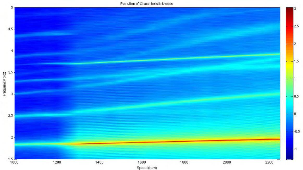
Figure 12: The variation of characteristic modes with rotation speed.
