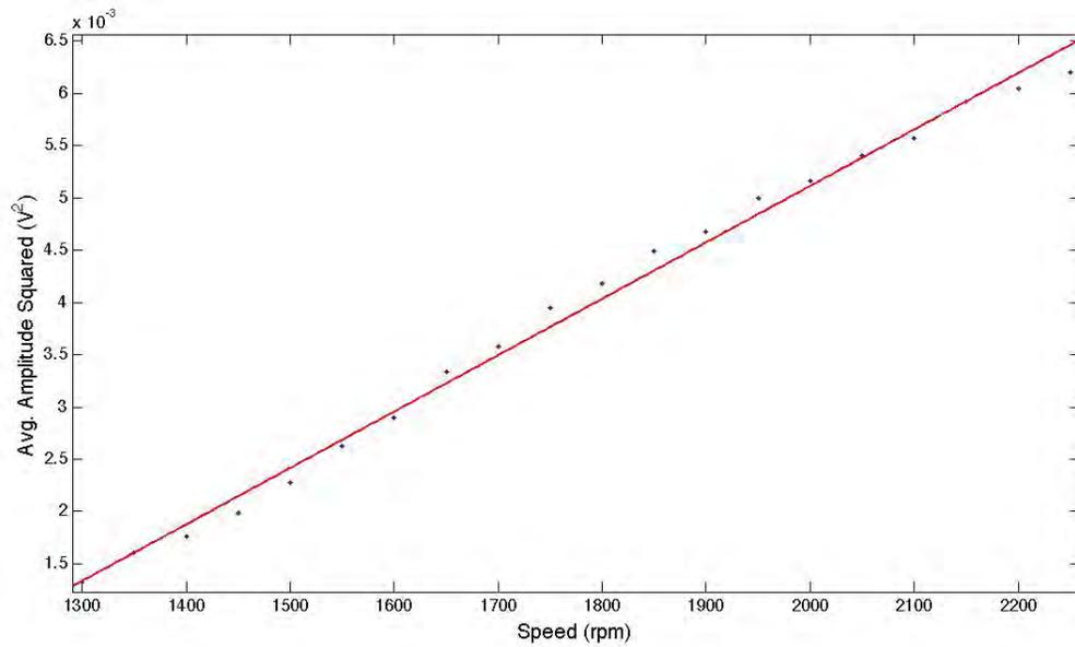
Figure 10: A plot of average amplitude squared vs. rotation speed. Linear correlation with  $R^2 = 99.3\%$
