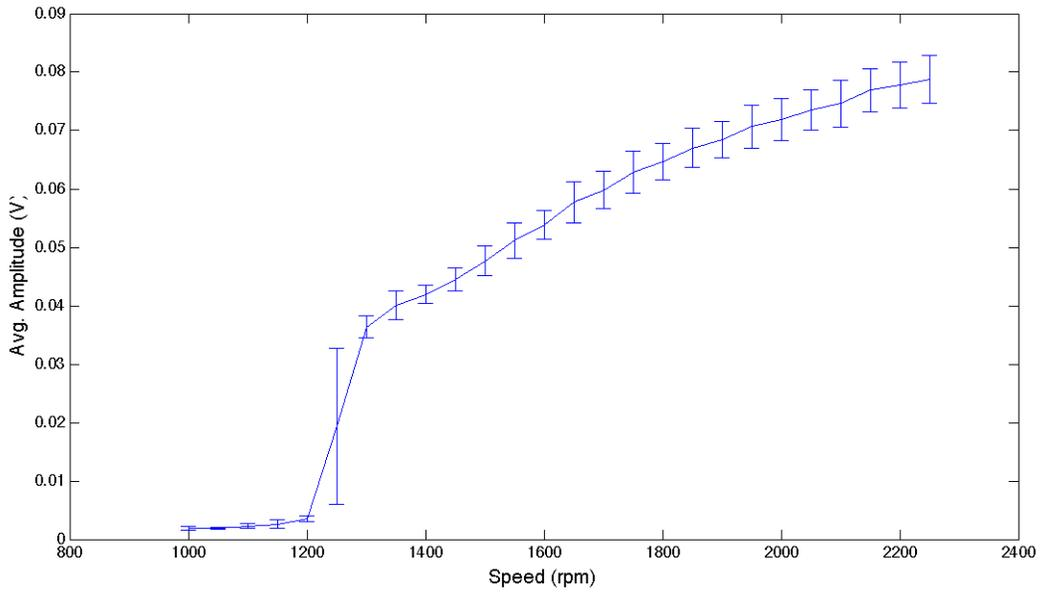
Figure 9: Bifurcation diagram of average wave amplitude vs. rotation speed.
