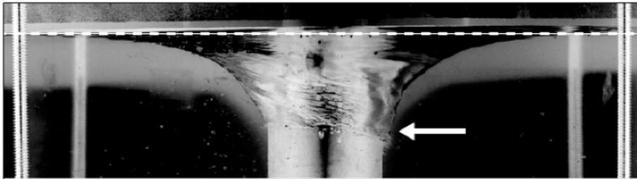
Figure 2: The ‘base state’ of Taylor-Couette flow. The slight asymmetry seen in this photo appears to undergo precession but time-averages to zero.
