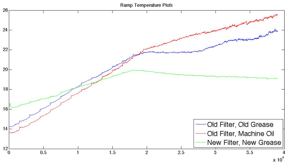
Figure 8: This graph shows the drastic improvement in temperature performance as a result of my mechanical changes. While the total net temperature change for runs of the old setup which were  $9.61^{\circ}\text{C}$  and  $11.95^{\circ}\text{C}$ , respectively, the total net change for runs of the new setup was  $2.93^{\circ}\text{C}$ , and improved even further during later runs as the apparatus settled.
