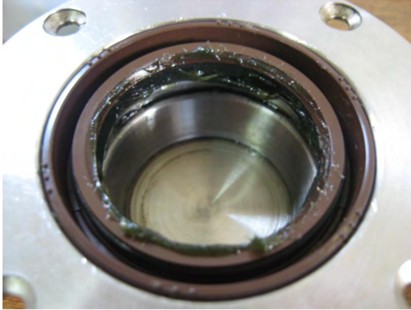
Figure 7: The new seal coated with new grease and mounted in the base. The new seal was able to withstand prolonged ramps without any damage.
