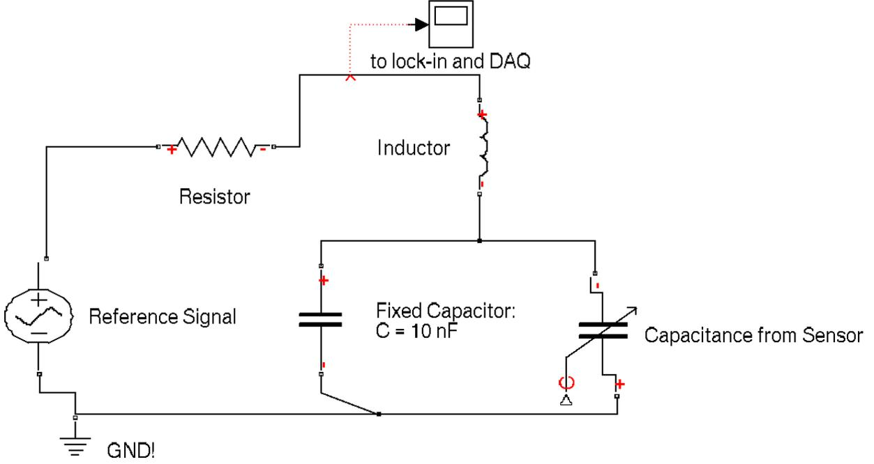
Figure 4: Resonant Circuit Diagram
