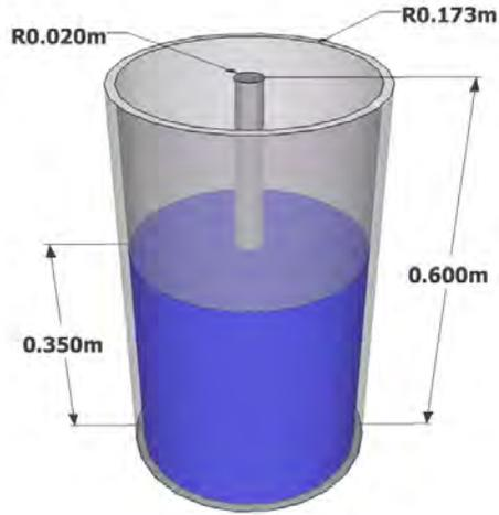
Figure 1: The main mechanical components of the system
