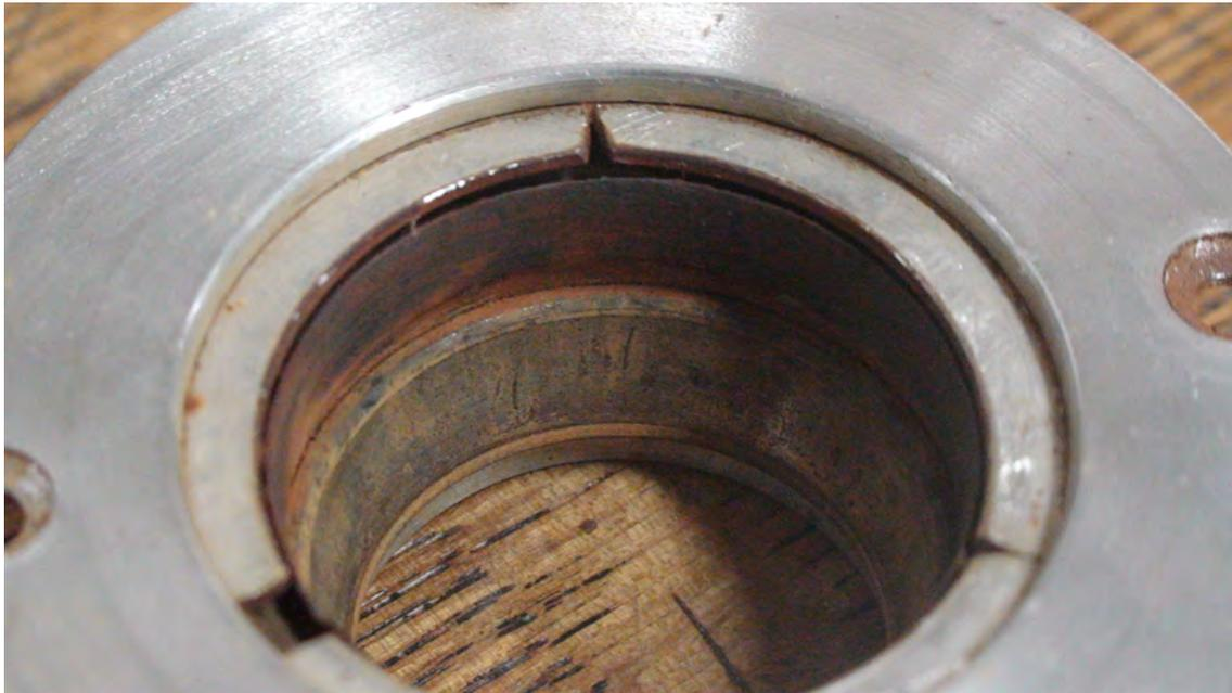
Figure 5: Interior base containing the graphite-teflon seal and rusted bearings after a trial run.
