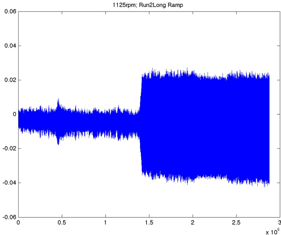
Figure 13: Data from an eight hour ramp, showing the wave appearing after 4 hours of running.
