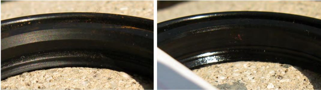
Figure 6: At left, the *nitrilo* seal before use. At right and after use, the degradation of the sealing (upper) lip is clear.
