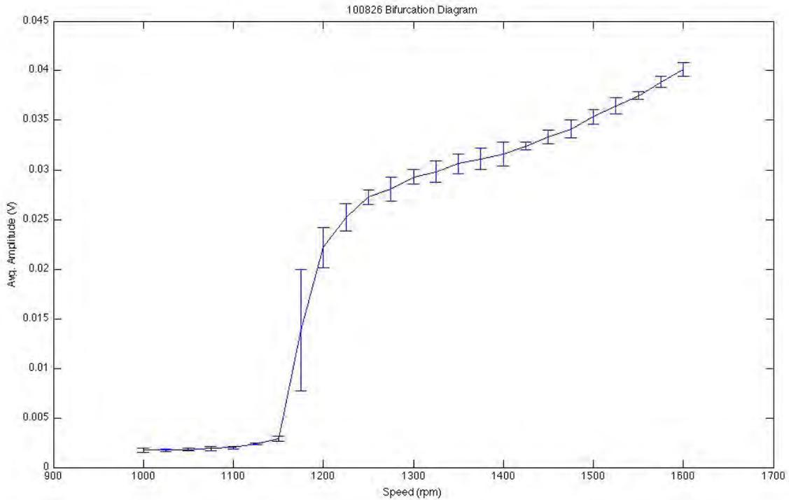
Figure 11: The bifurcation diagram after disassembling and re-assembling the system, showing bifurcation around 1175 rpm.
